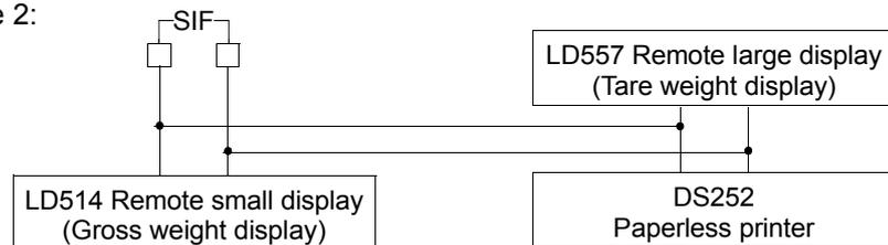
These indicated above are examples for the connection of Remote small displays, Remote large display and printer. Each display and printer can select the data individually.
