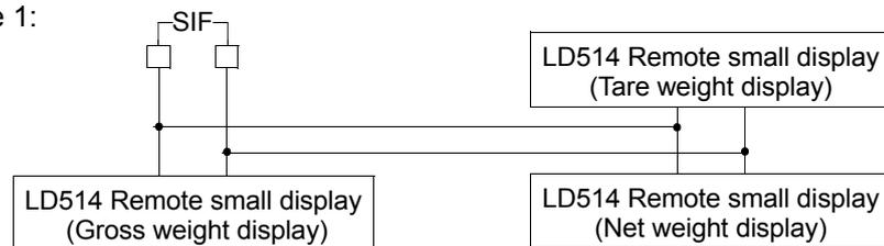
Up to 3 remote small displays can be connected. The each display can display individual content according to the selection.
